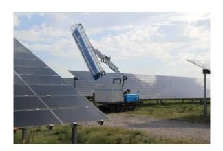
Guided by a sensor cleaning system prevents any impact on the panels and optimizes washing freeing itself from the constraints of terrain.
